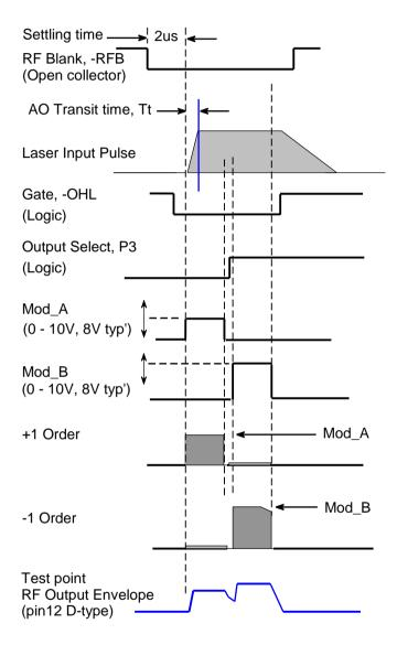
Logic levels are 5V-CMOS / TTL compatible, except -RFB
