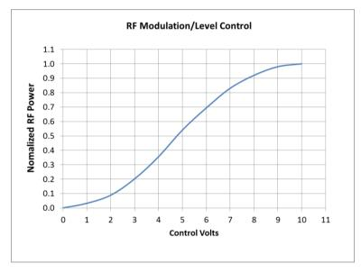
Typical RF power characteristic per output
