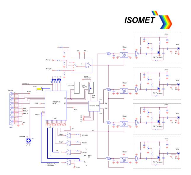
Figure 5: Driver Block Diagram
