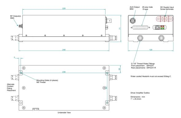
Figure 4: Driver Installation
