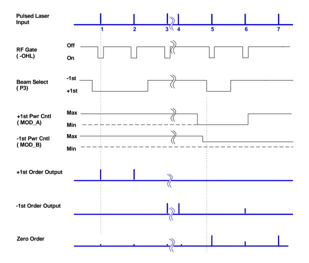
Logic levels are 5V-CMOS / TTL compatible except -RFB
