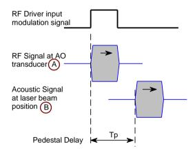
2: Transit time = time for the acoustic wavefront to cross the laser beam.
