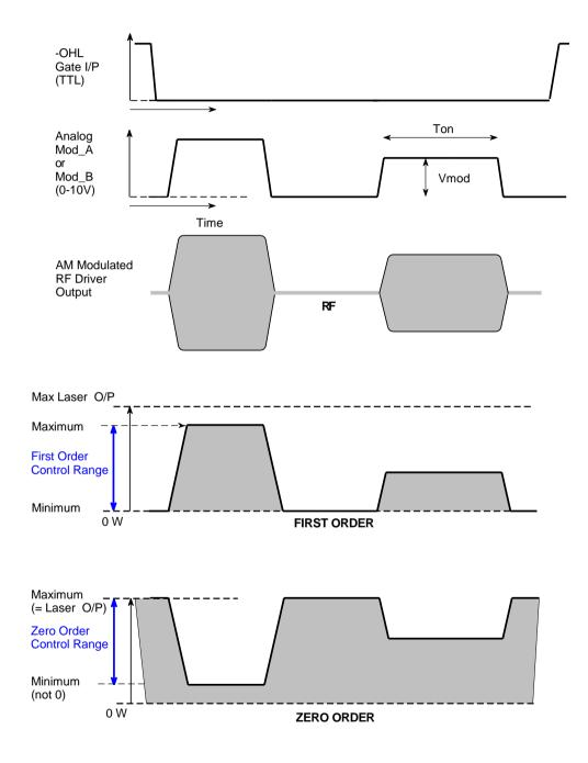
Figure 2: Typical Laser Modulation Waveforms
